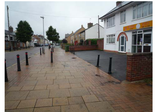
"A" boards and bollards are an issue to visually impaired
